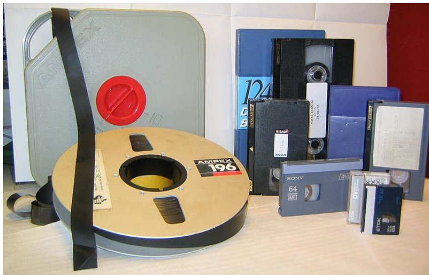
Figure 2.3 – Examples of magnetic tapes used for video recording [7]
